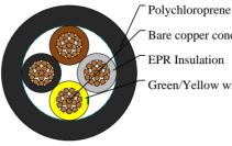
Polychloroprene rubber outer jacket Bare copper conductor EPR Insulation Green/Yellow wire
